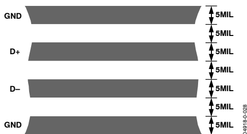
Figure 29. Arrangement of Signal Tracks
